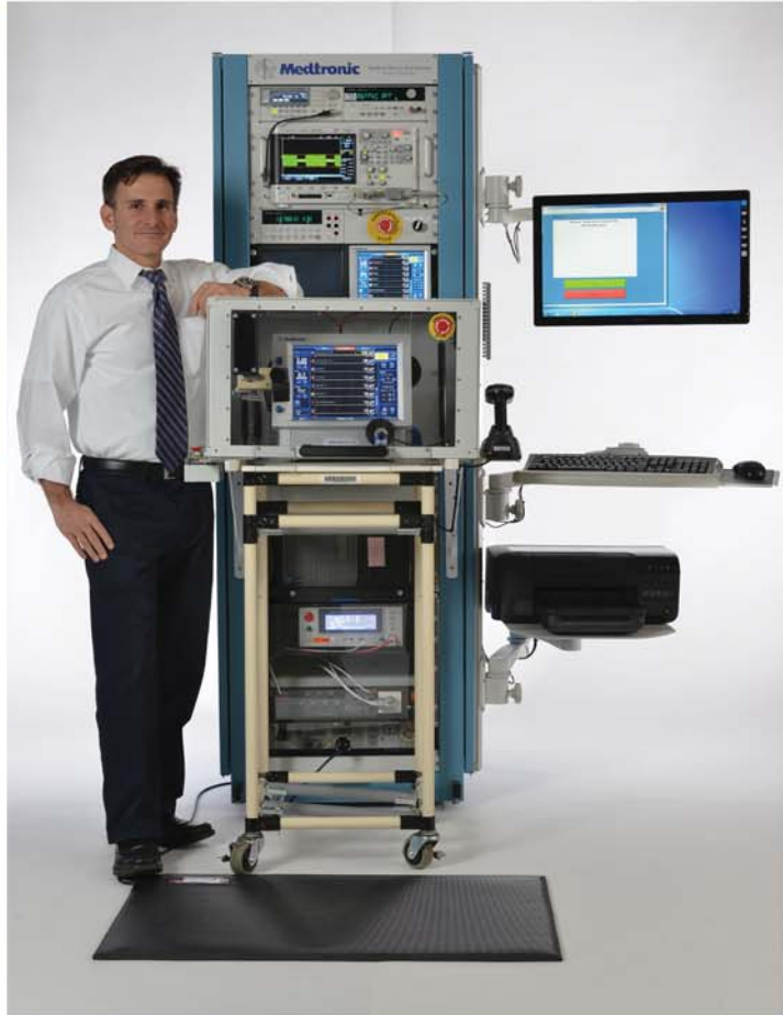
Front view of Tester with HIPOT and Safety Mat
