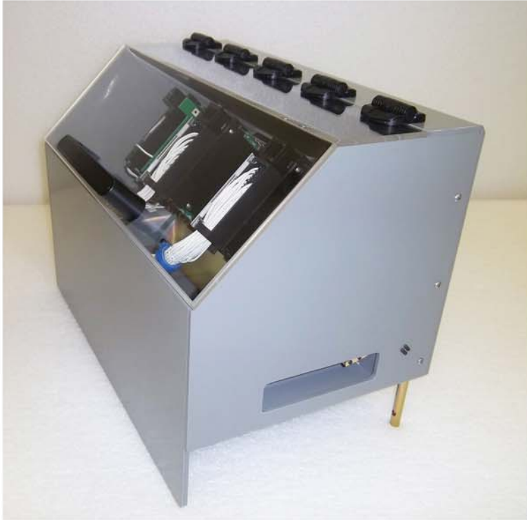
Programmable Logic Card Hipot Fixture
