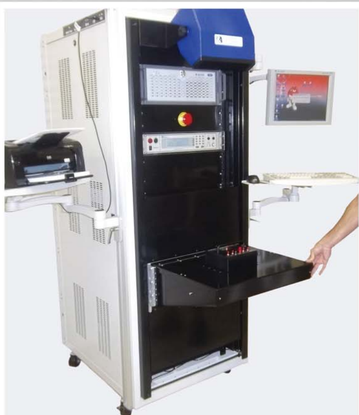
Ergonomic Hydraulic Table Top adjusts Up/Down
