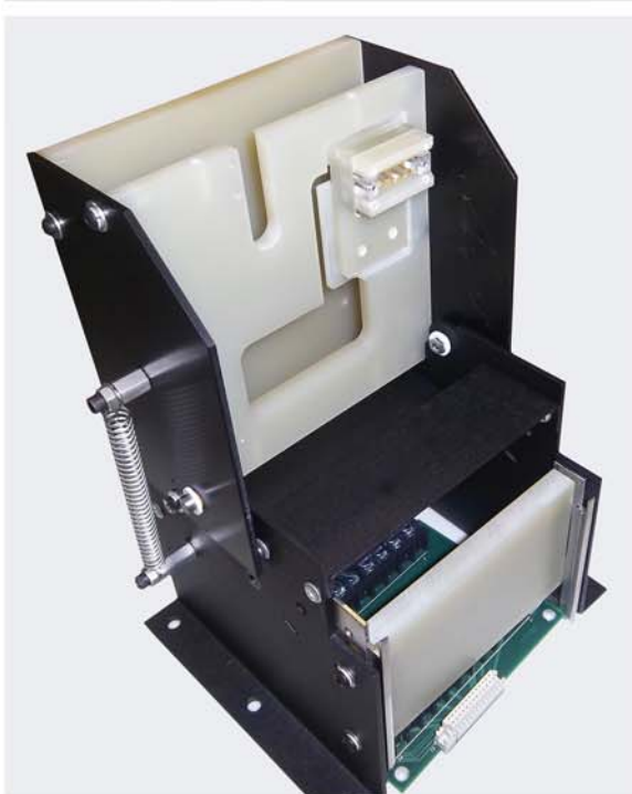
Mechanical Mechanism with Pogo-Pin Connections to UUT
