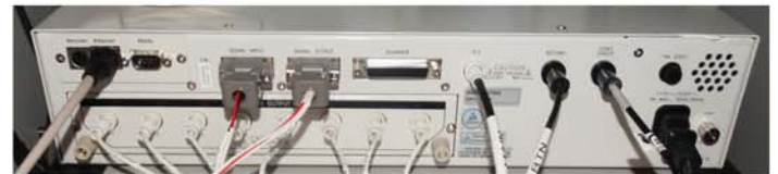
Rear view of Hipot with built-In 8x1 HV Mux
