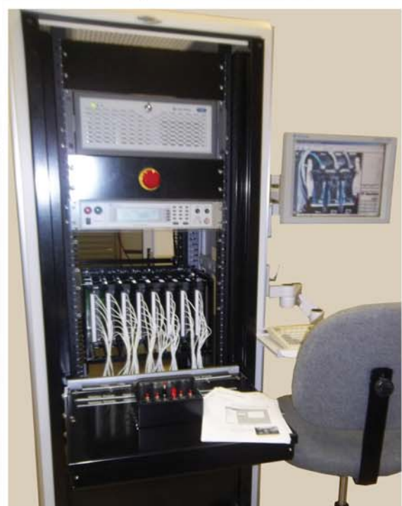
Open View Dual 64x1 HV Mux
