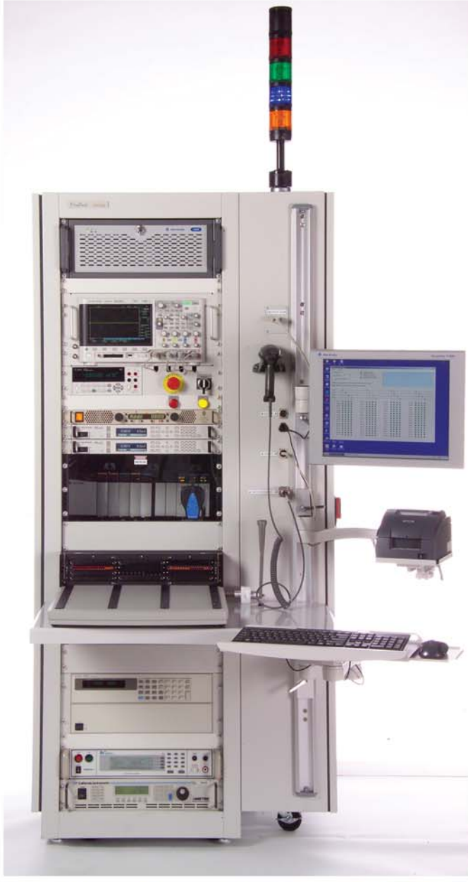
Front view of Tester with Integrated HIPOT
