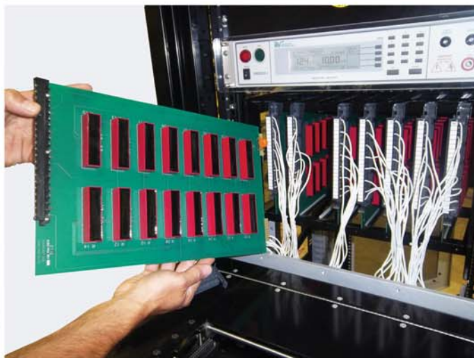
Close-Up of Dual 8x1 HV Mux Card
