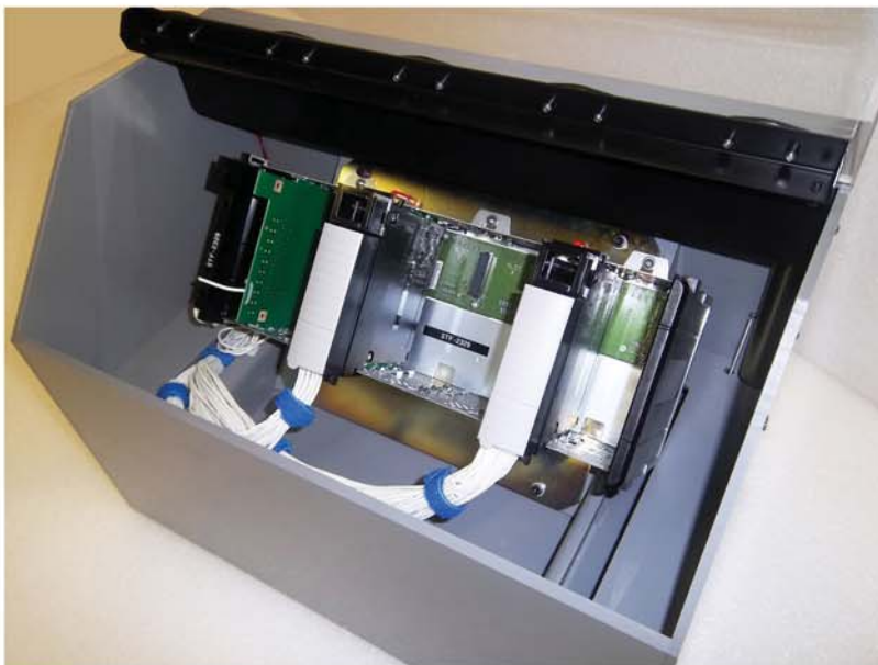
Inside View showing end product mounting rack with UUTs installed
