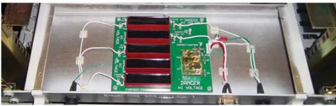
Close-Up FineTest HV Relay Unit for Hipot
