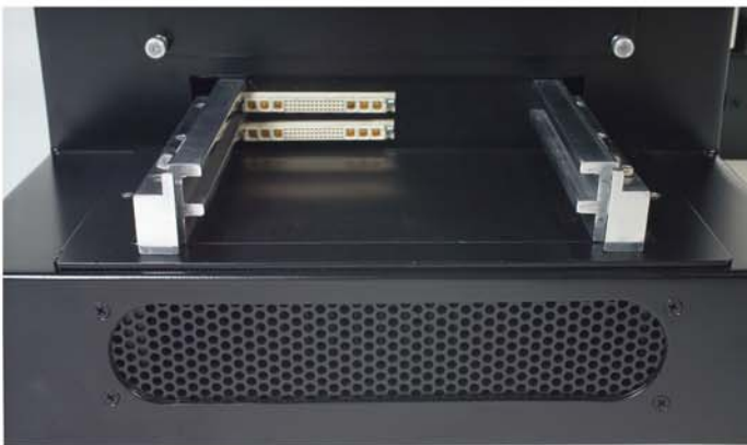
Dual Insertion Test Fixture: One for Hipot and one for Functional Test
